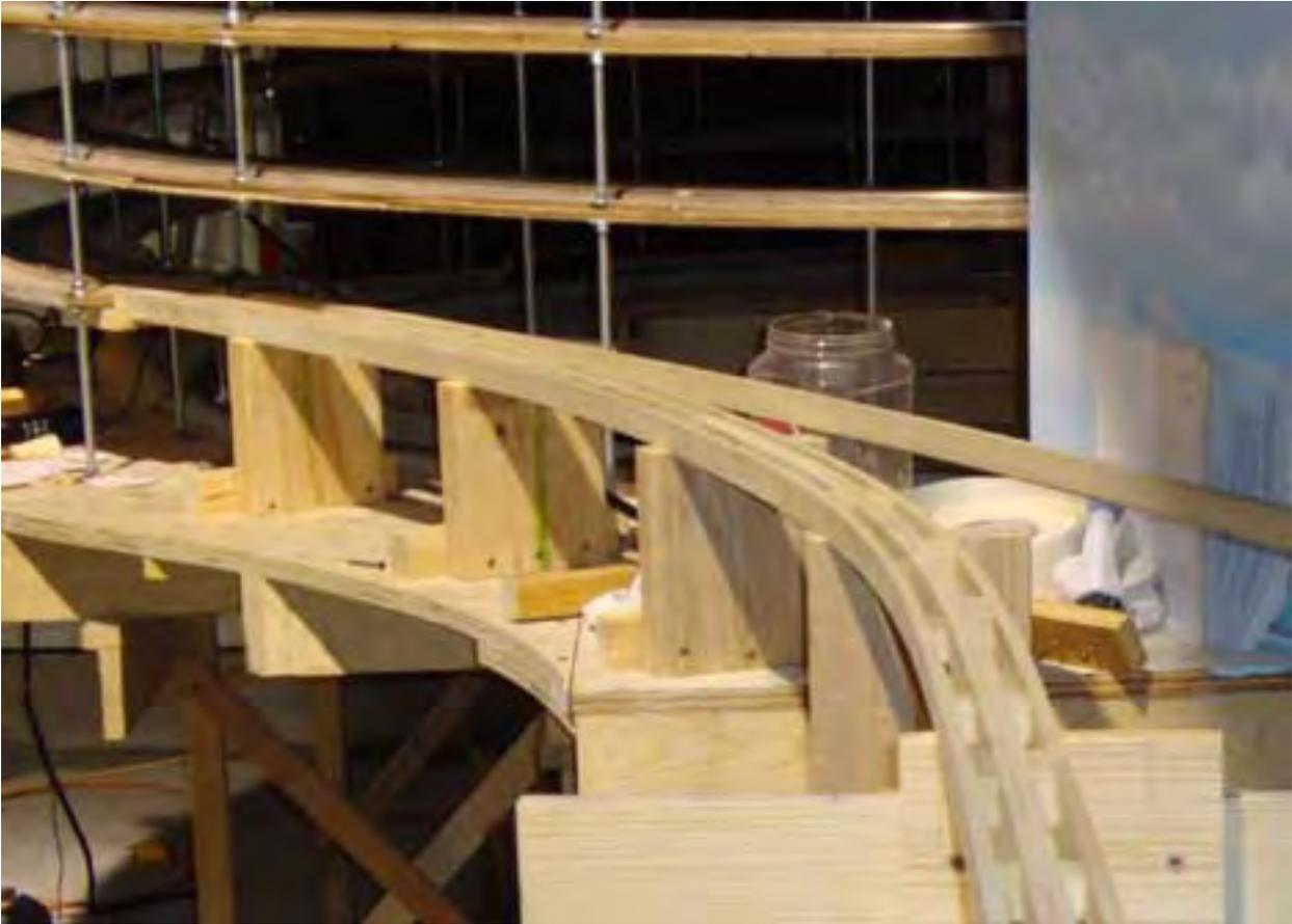
The spacers were glued to the backbone, the outside layer of the spline has been glued to the spacers, and this is the beginning of the lower outside main line.
