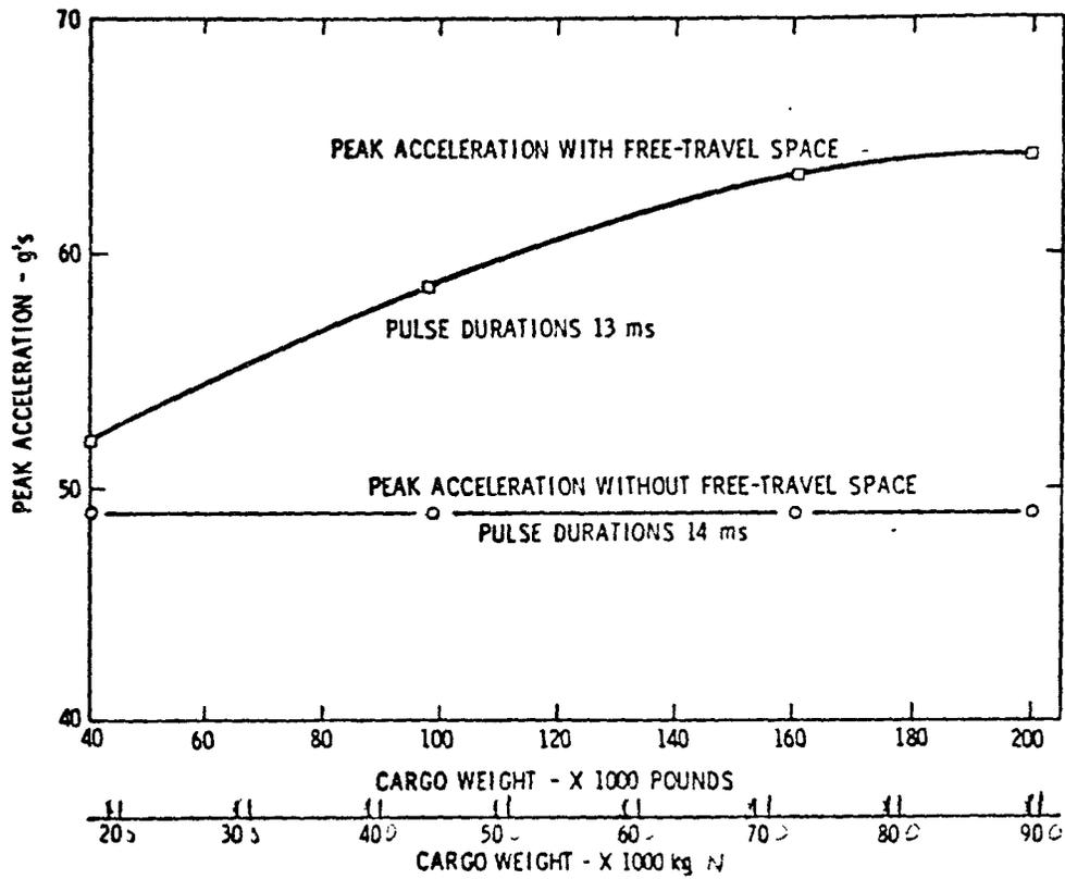
Figure 3. Peak Acceleration and Pulse Duration Half-Sine Pulses - Spent Fuel Cask System Longitudinal Axis.
