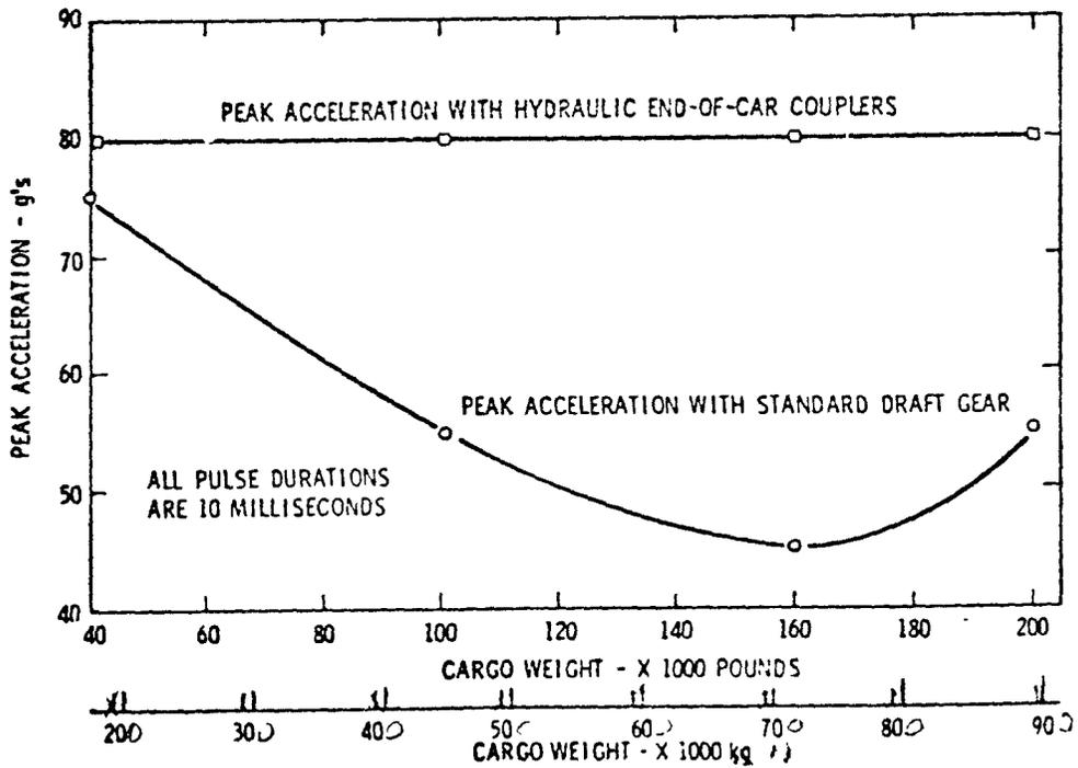
Figure 4. Peak Acceleration and Pulse Duration Half-Sine Pulses - ATMX System Longitudinal Axis.
